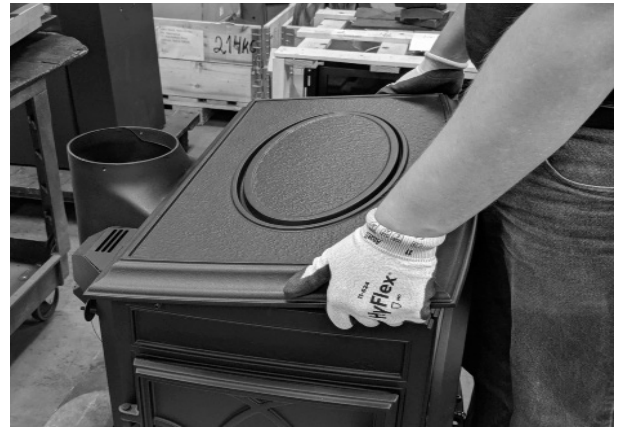
Fig. 21. Remove the top plate from stove.
